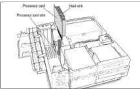
Installing the MACh Speed G3 Upgrade Card
